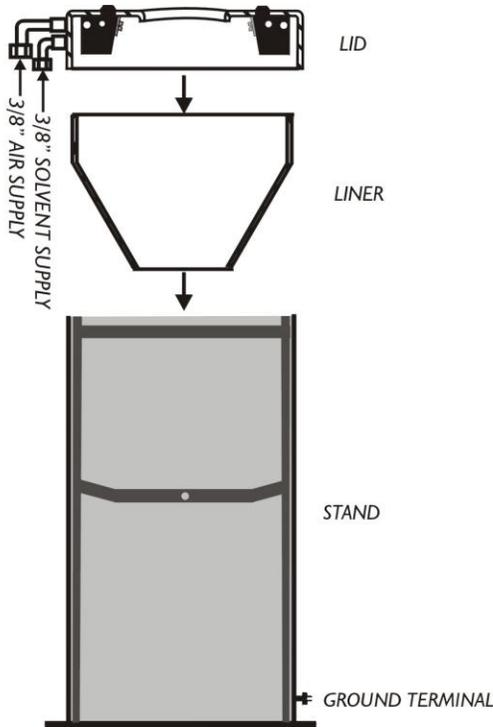
Connect a 3/8" (10mm) air supply line from the three-way regulated air valve to the uppermost line on the cleaner. Set the air pressure to 45 psi (3 Bar)\*.
